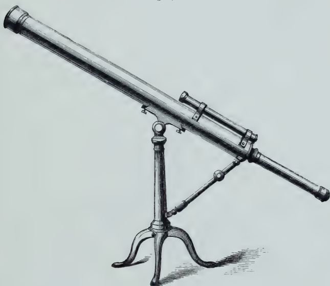
TELESCOPE MOUNTED ON PILLAR-AND-CLAW STAND, WITH FINDER AND VERTICAL RACK MOTION.
